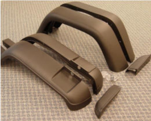
The flare kit includes: 1 each of Left and Right front flares (2 front extensions if ordered), Left and Right rear flares, and the required hardware to install the flares.
