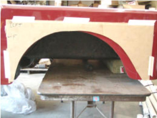
Only the rear half of the YJ wheel opening needs to be enlarged. Notice the large amount of added clearance the new flare will provide. Mark the area and cut as required.
